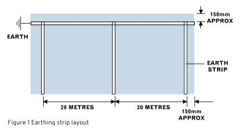
Further strips are laid at 20 meter intervals as determined by the size of the room.
